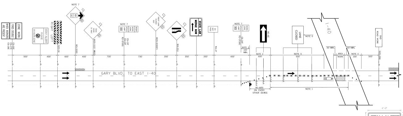
MAXIMUM SPACING BETWEEN CHANNELIZING DEVICES (FEET) SHALL BE TWICE THE POSTED SPEED LIMIT (M.P.H.) WITH THE FOLLOWING EXCEPTIONS, SPACING SHALL NOT EXCEED 50 FEET FOR CONES OR TUBE CHANNELIZERS. SPACING SHALL NOT EXCEED 75 FEET FOR CHANNELIZER CONES. SPACING SHALL NOT EXCEED 100 FEET FOR TYPE II BARRICADES, VERTICAL PANELS
